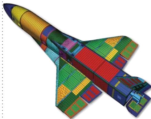
▲ Finite element analysis model of the X-34
